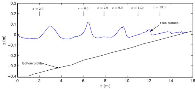
**Fig. 6.** Definition sketch for Ting and Kirby (1994) spilling breaking experiment,  $H_0=0.127$  m,  $L_0=3.74$  m, and  $T=2.0$  s (computed results using the proposed breaking model). Vertical lines correspond to locations of wave gauges in meters.
