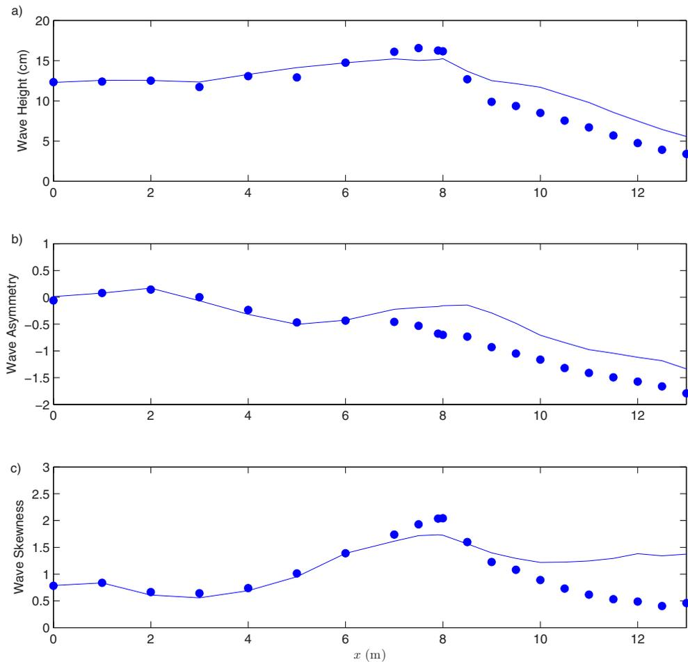
**Fig. 2.** Comparison between measured (●) and computed (—) wave properties for Ting and Kirby's (Ting and Kirby 1994) spilling breaking experiment using Kennedy et al. (2000) parameterization with  $\delta_b=1.2$ . (a) Wave height; (b) wave asymmetry; and (c) wave skewness.
