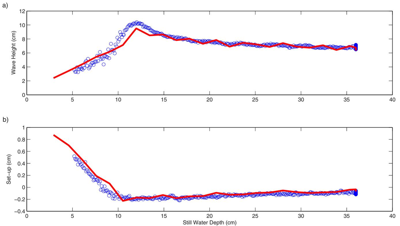
**Fig. 12.** Comparisons of model predictions and experimental data for Hansen and Svendsen (1979) spilling breaking test No. 061071. (○): measured data. Computed wave height and setup are plotted in solid lines.
