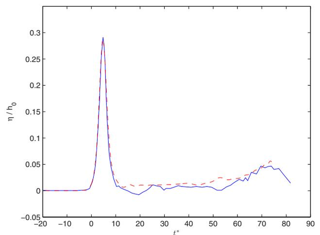
**Fig. 16.** Computed and measured incident and reflected solitary wave for the breaking case with  $a_0/h_0=0.28$  investigated by Synolakis (1987). Wave gauge located 4.775 m from the still shoreline and  $t^* = t\sqrt{g/h_0}$  is the nondimensional time. (—) measured time series, and (---) predicted one using the numerical model.
