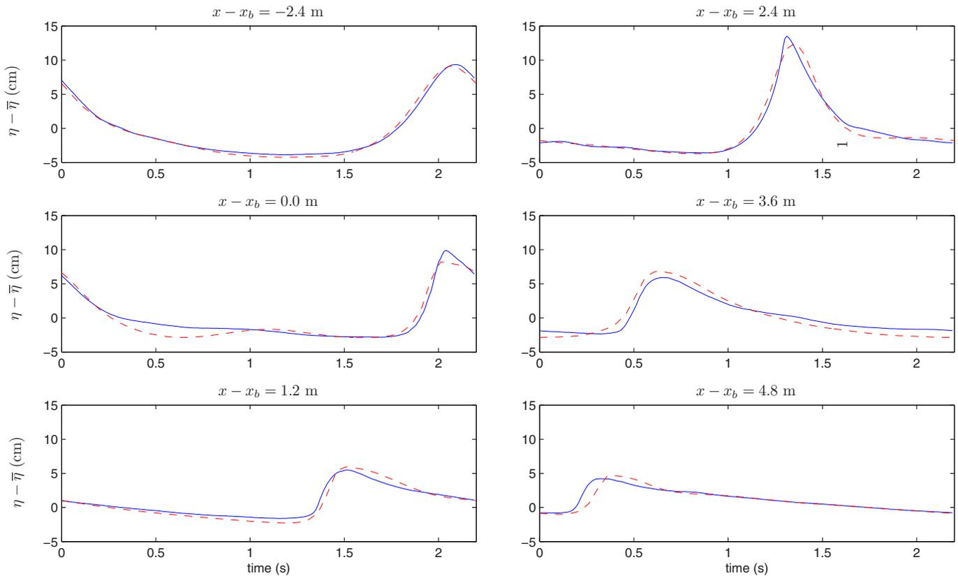
**Fig. 10.** Computed and measured phase-averaged time series of free-surface elevation at several wave gauges for Cox (1995) experiment.  $x_b$  is the coordinate for breaking initiation. (—): measured and (---) computed.
