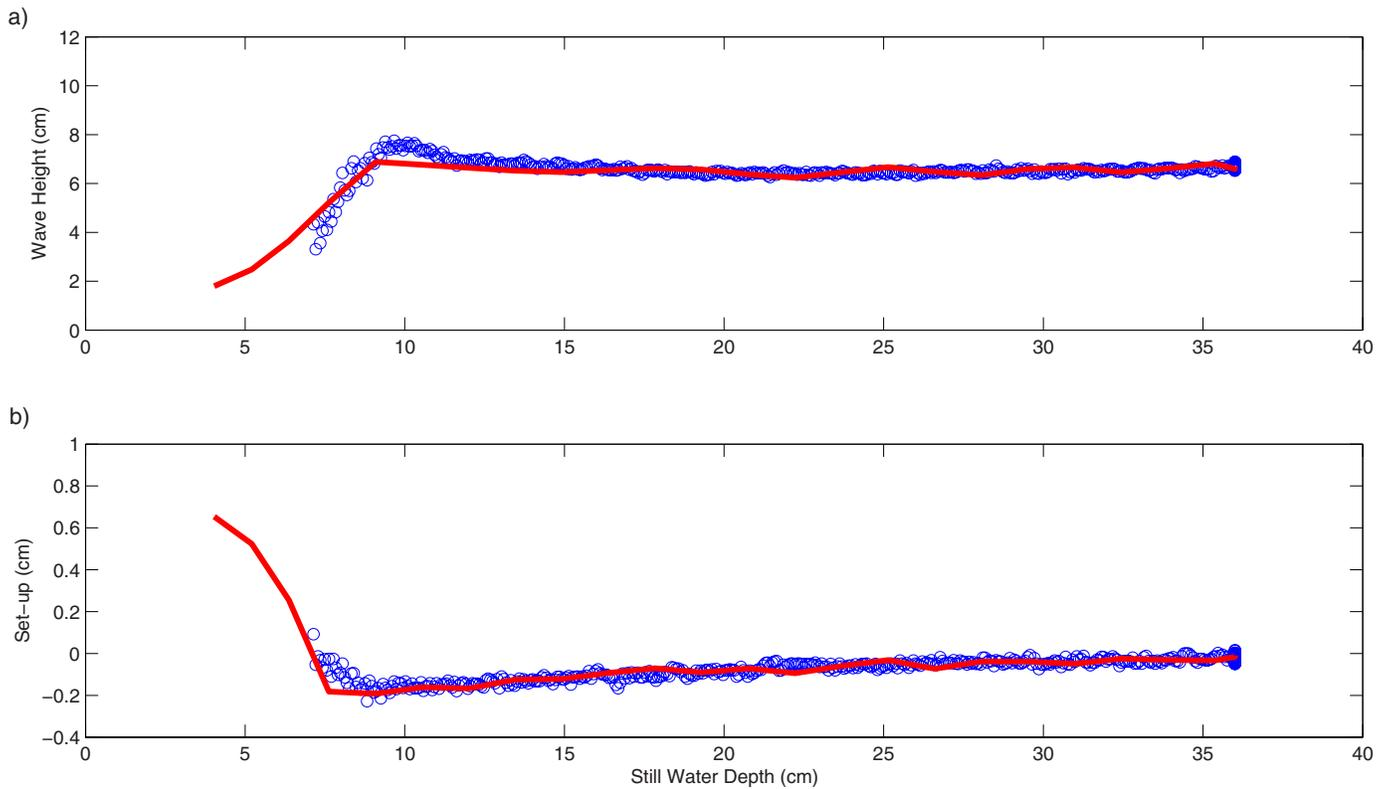
**Fig. 11.** Comparisons of model predictions and experimental data for Hansen and Svendsen (1979) spilling breaking test No. A10112. (○): measured data. Computed wave height and setup are plotted in solid lines.
