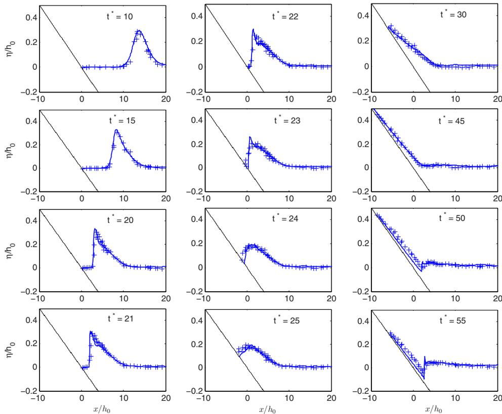
**Fig. 17.** Comparisons of model predictions and experimental spatial snapshots for the breaking solitary wave with  $a_0/h_0=0.28$  investigated by Synolakis (1987). (+): experimental data, while numerical results are plotted in solid lines.  $t\sqrt{g/h_0}$  is the nondimensional time.
