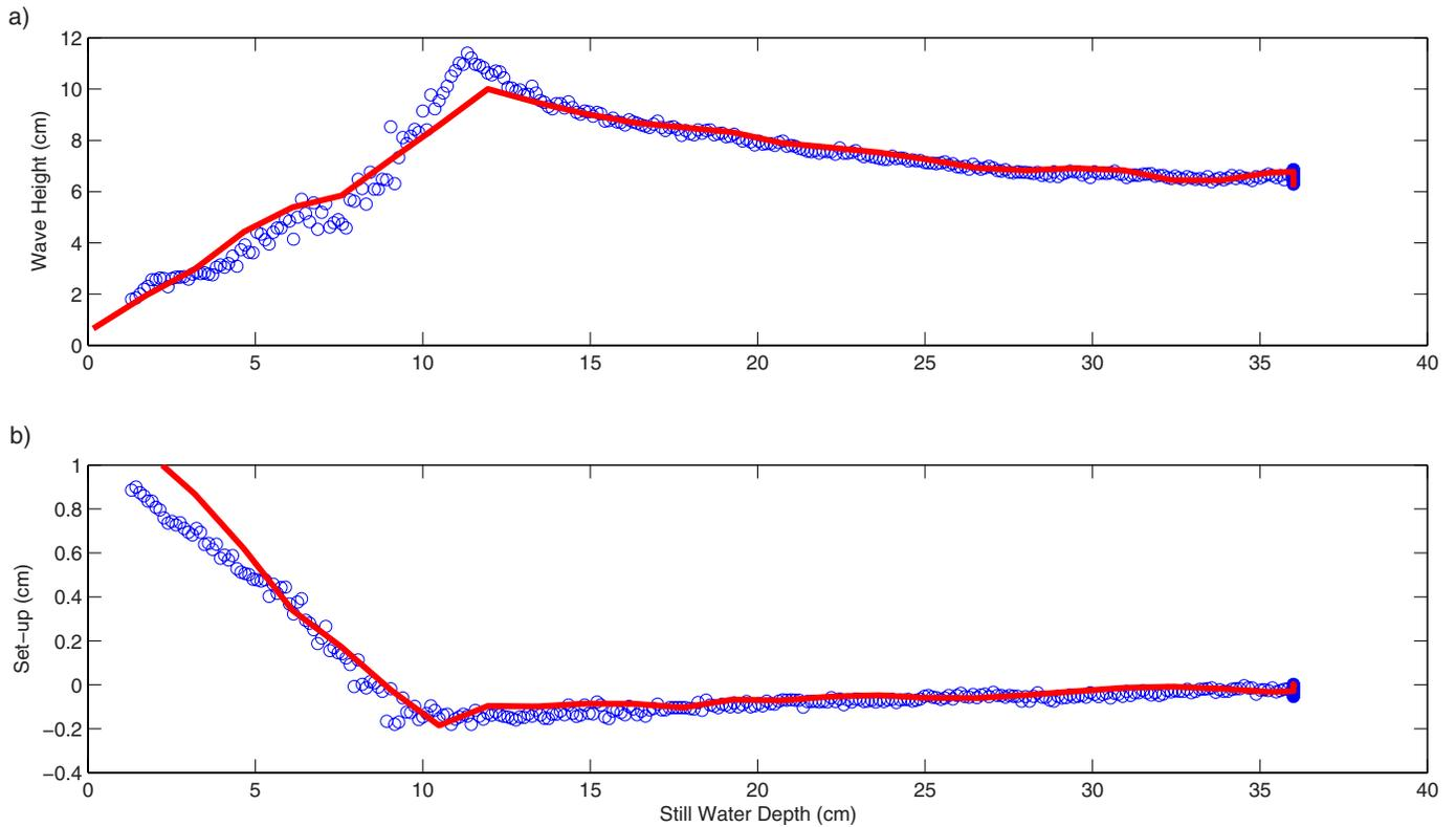
**Fig. 13.** Comparisons of model predictions and experimental data for Hansen and Svendsen (1979) spilling breaking test No. 053074. (○): measured data. Computed wave height and setup are plotted in solid lines.
