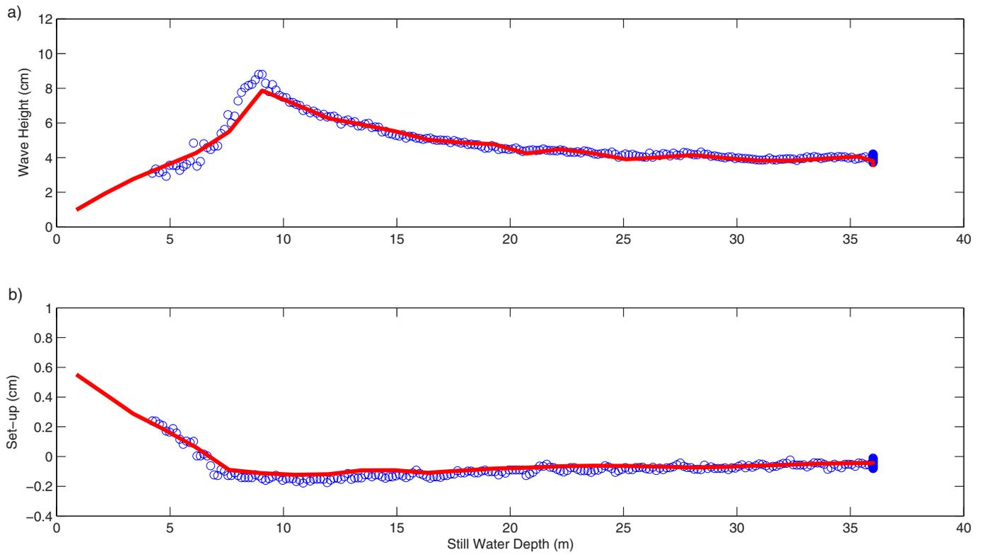
**Fig. 14.** Comparisons of model predictions and experimental data for Hansen and Svendsen (1979) plunging breaking test No. 041041. (○): measured data. Computed wave height and setup are plotted in solid lines.
