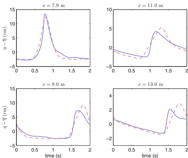
**Fig. 3.** Computed and measured phase-averaged time series of free-surface elevation for Ting and Kirby (1994) spilling breaking experiment at several wave gauges using Kennedy et al. (2000) parameterization with  $\delta_b=5.5$ . (—): measured; (---) computed
