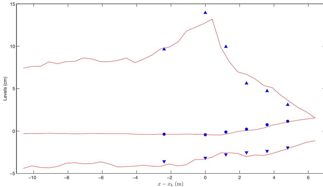
**Fig. 9.** Comparisons of model predictions and experimental data for Cox (1995) spilling breaking,  $H_0=0.115$  m,  $L_0=4.19$  m,  $T=2.2$  s. ( $\blacktriangle$ ): measured crest level  $\eta_c - \bar{\eta}$ ; ( $\bullet$ ): measured wave-averaged free surface  $\bar{\eta}$ ; ( $\blacktriangledown$ ): measured trough level  $\eta_t - \bar{\eta}$ . Computed properties are plotted in solid lines.
