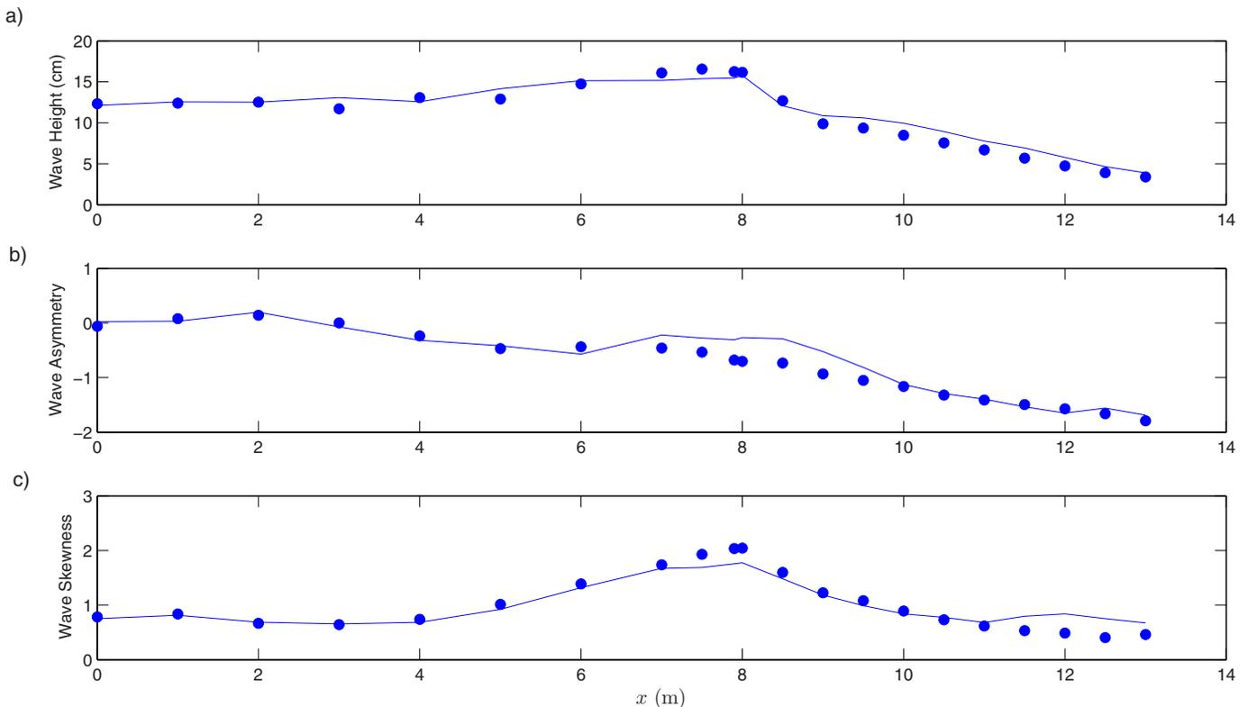
**Fig. 8.** Comparison between measured (●) and computed (—) wave properties for Ting and Kirby (1994) experiment using the proposed breaking model. (a) Wave height; (b) wave asymmetry; and (c) wave skewness.
