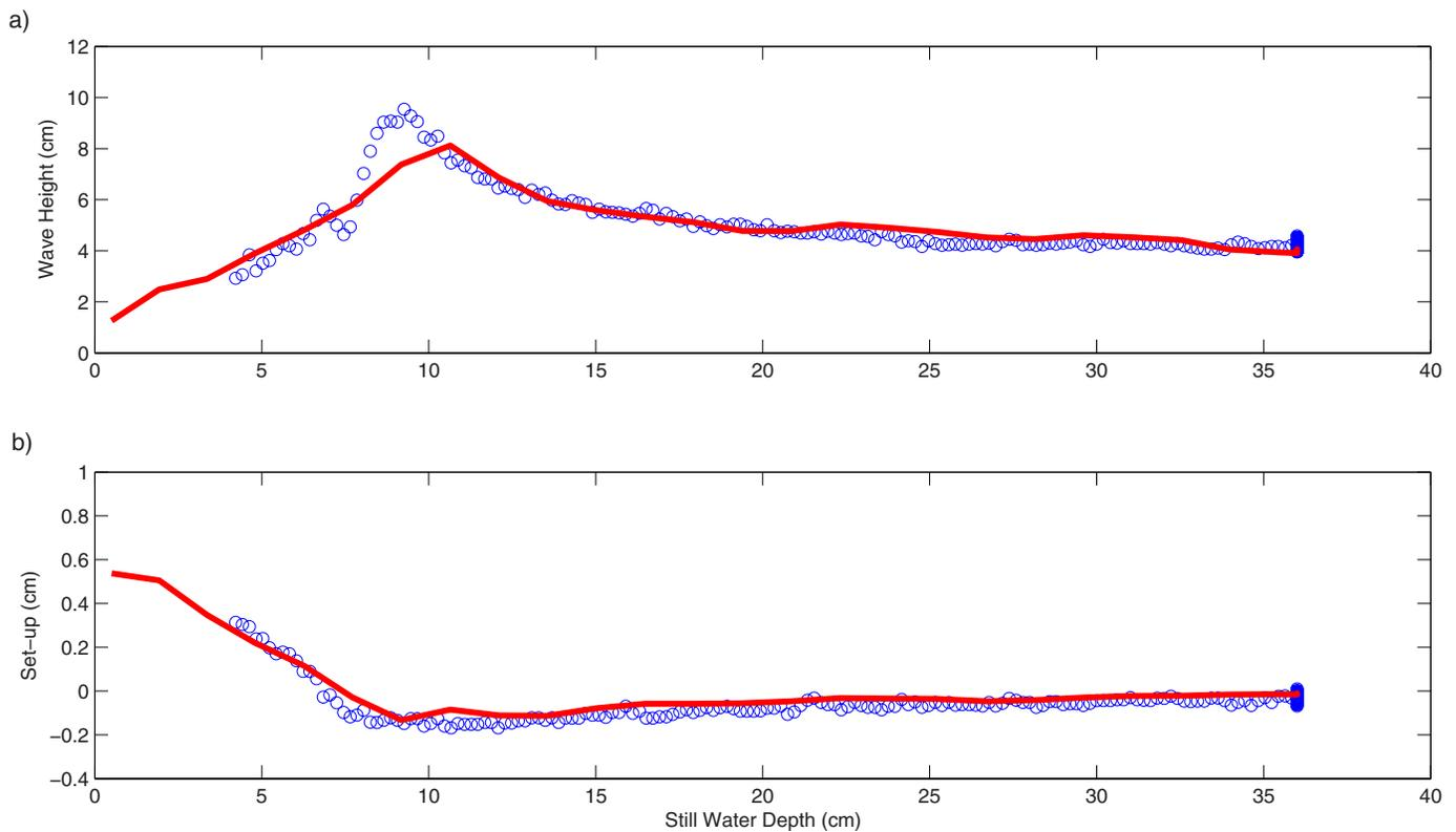
**Fig. 15.** Comparisons of model predictions and experimental data for Hansen and Svendsen (1979) plunging breaking test No. 031041. (○): measured data. Computed wave height and setup are plotted in solid lines.
