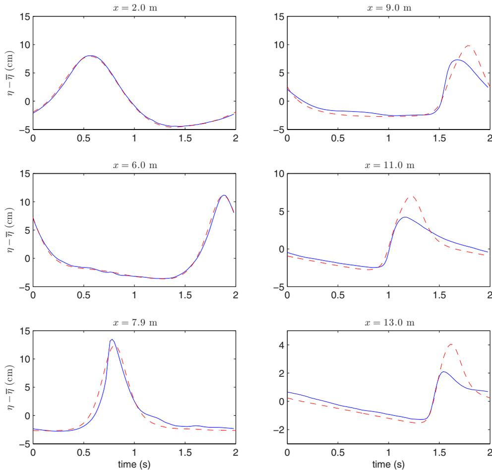
**Fig. 1.** Computed and measured phase-averaged time series of free-surface elevation for Ting and Kirby (1994) spilling breaking experiment at several wave gauges using Kennedy et al. (2000) parameterization with  $\delta_b = 1.2$ . (—): measured; (---) computed
