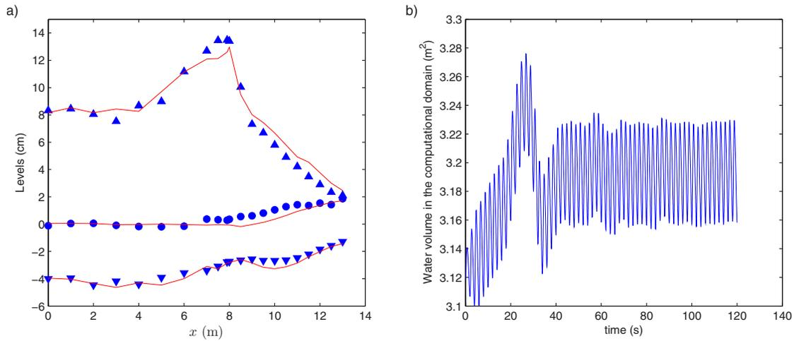
**Fig. 7.** Numerical predictions for Ting and Kirby (1994) spilling breaking experiment using the proposed breaking model. (a) (▲): measured crest level  $\eta_c - \bar{\eta}$ ; (●): measured wave-averaged free surface  $\bar{\eta}$ ; (▼): measured trough level  $\eta_t - \bar{\eta}$ ; computed properties are plotted in solid lines; (b) temporal evolution of the water volume contained in the numerical domain.
