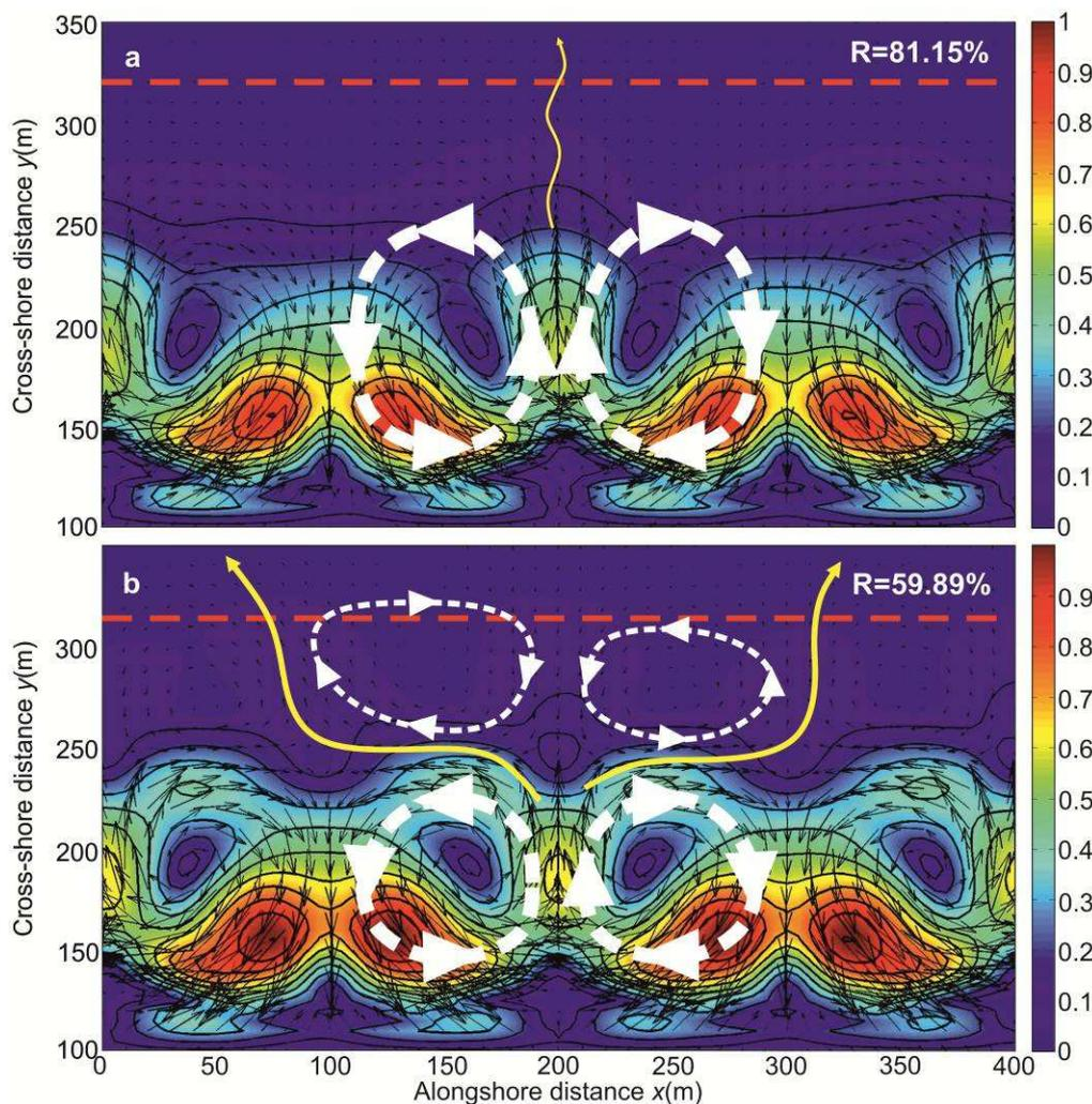
Figure 4. Computed mean flow patterns (for clarity one out of two vectors are plotted in both directions) and surfzone retention  $R$ . Colorbar indicates mean flow velocity in m/s. The dotted white circles and yellow arrows indicate qualitatively the surf zone eddies and the preferred pathways of drifter exits. (a) Reference case simulation and (b) simulation with the presence of a well-developed rip head bar with  $Arhb = 0.4$  m.
