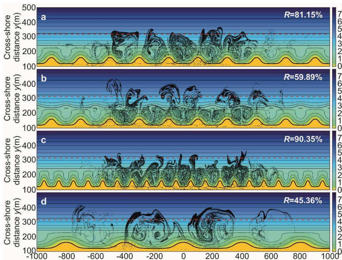
Figure 5. Snapshot of drifter positions (black dots) at  $t = 60$  min and resulting hourly retention rate  $R$  for (a) the reference case simulation (b) adding a rip head bar with  $Arhd = 0.4$  m and with different spacings (c)  $\lambda = 100$  m and (d)  $\lambda = 400$  m. In all panels, surf zone compartment is indicated by the dashed red line and iso-contours (0.5-m intervals) are contoured in the background. Colorbars indicate still water depth in meters.
